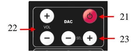
(\*) *Volume control is possible only with By-Pass Off. When changing the volume, level shows shortly on display, then the display shows the sampling frequency.*
